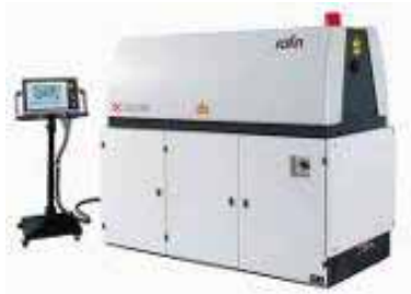
Diffusion-Cooled CO 2 -Laser 1,000 – 8,000 W
