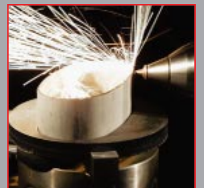
Cutting with diode pumped, solid-state laser
