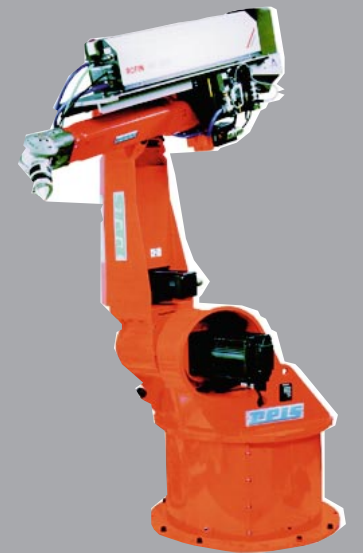
Sealed-off laser mounted on a robot
