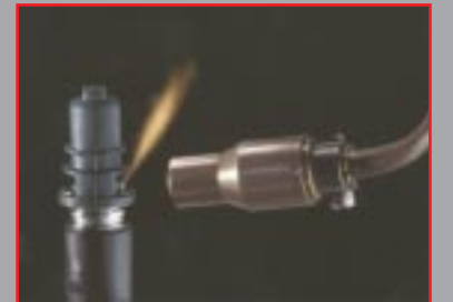
Welding of injection nozzles
